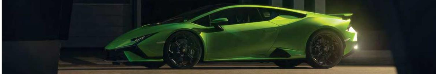
The Tecnica lacks the STO's wild aerodynamic add-ons but a big new rear wing helps to contribute 35% more downforce than the Evo RWD, at the same time delivering 20% less drag. A unique rear end features a 61mm longer tail than the Evo, with a lengthened glasshouse inspired by Lamborghini's Essenza SCV12. High-exit hexagonal exhaust tailpipes are flanked by large apertures beneath contoured tail-lights. An all-new carbonfibre engine cover sits flat to improve visibility.
