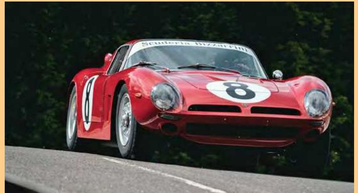
For racing, the GT Corsa uses a single-piece composite body over a steel frame with a six-point rollcage and safety fuel cell that meet FIA Historic Racing regulations. A full carbonfibre bodysell will be offered to those customers who do not wish to race in Historics. The 5300cc V8 engine uses Weber 45 DCOE carburettors to develop over 400hp, giving the 1250kg car a strong power-to-weight ratio. 24 examples of the Revival will be built, with the first deliveries scheduled for May 2022.
